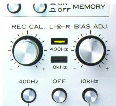
Fine-bias adjustment optimizes the characteristics of each individual tape.
